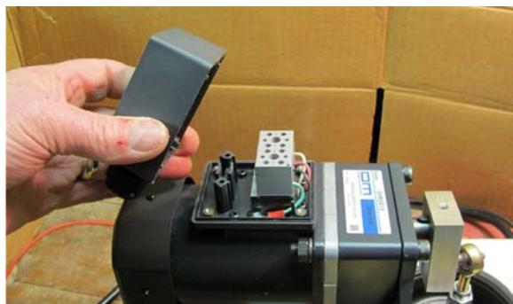
Figure 5. Remove junction box cover.
