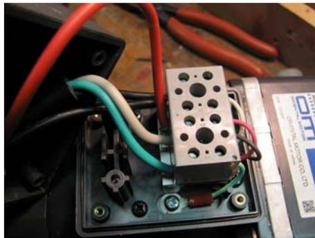
Figure 16. Connect black wires to Z2.
