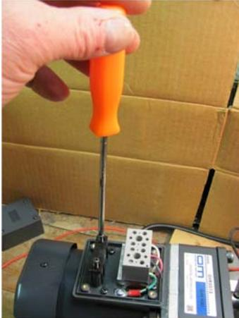
Figure 6. Remove strain relief strap.
