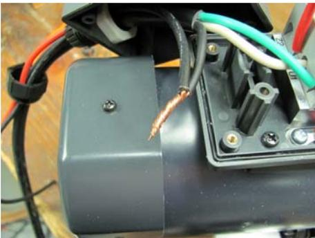
Figure 15. Twist black wires together and cut to 1/2".
