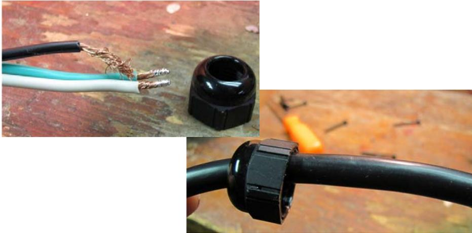
Figure 9. Thread power cord through wire nut.
