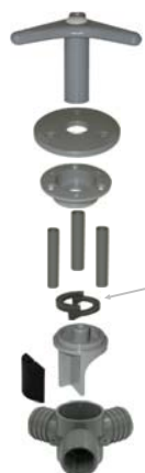
Easily removable travel stop ring converts from 2 flow-path mode to 3 flow-path mode
