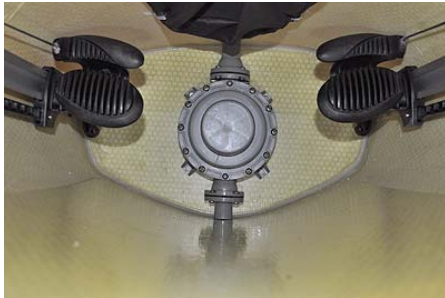
Guzzler GF-0400D foot pump mounted to kayak bulkhead bracket. (Image courtesy of Hybrid Pty Ltd.)
