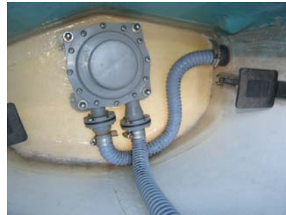
Kayak installation of Guzzler GF-450D foot pump with same-side ports
