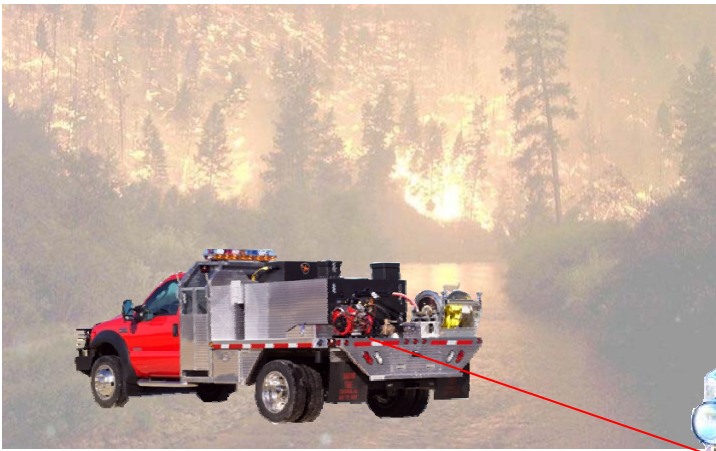
Guzzler priming fire-safety pumps in truck slip-on unit
